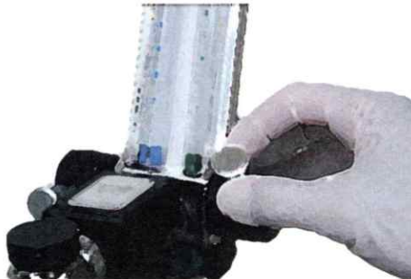
Step 5: Adjust O 2 (oxygen) flow rate to desired level.
