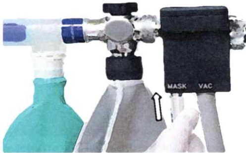
Step 3: Connect the end of the NITROUSEAL Circuit exhalation limb to the nipple marked "MASK" underneath AVS module.
