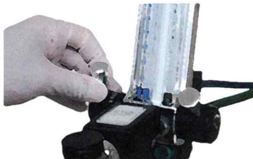
Step 7: Adjust N 2 O (nitrous) flow rate to desired level.
